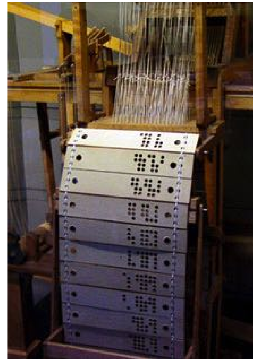
Jean-Baptiste Falcon: In 1728, replaced paper tape with cards connected to form an endless chain.
