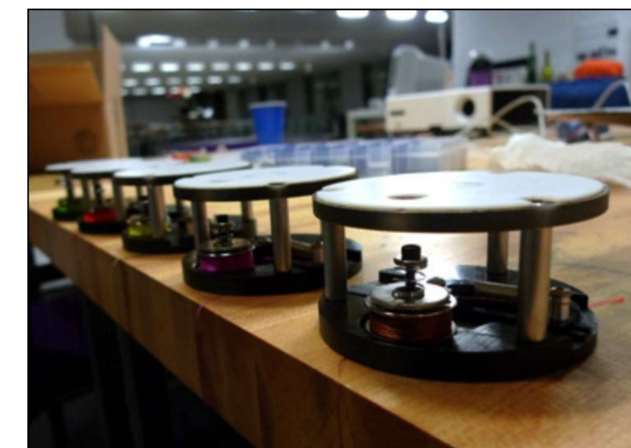
Different types and/or colors of thread are held in pucks.
