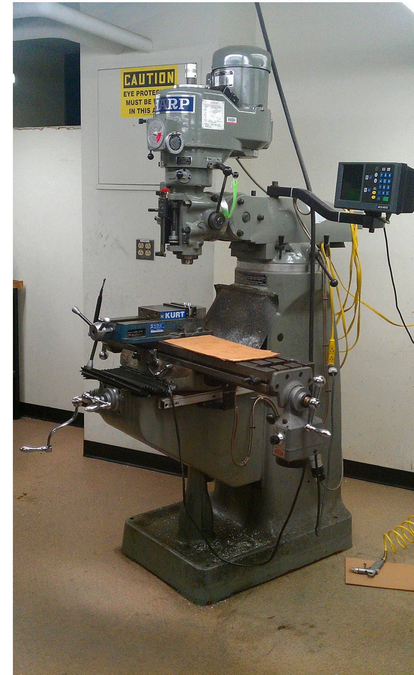
A 3-axis clone of a Bridgeport-style vertical milling machine
